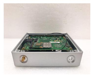
Step 4 Put the washer and Hex nut into the antenna cable connector, and tighten it up.
