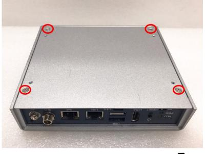
Step 3 Remove the bottom cover, and locate MicroSD icon **D** on the board.
