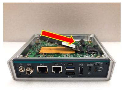
Step 7 Press it down gently, but firmly, and then secure the M.2 2280 Key M SSD drive to the carrier by tightening up the one M3 Phillips head screw to the marked position.
