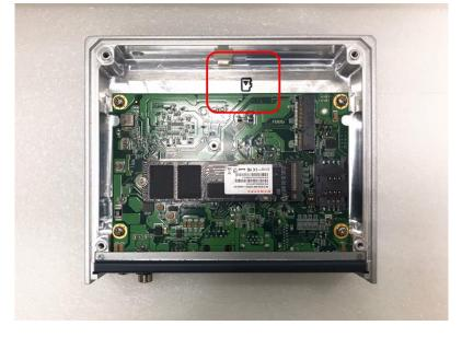
Step 4 Turn the MicroSD card upside down, and hold it with fingers at a 30 degree angle up from horizontal, and then insert and press it gently.
