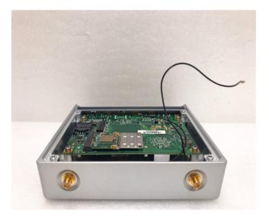
Step 5 Connect the antenna cable to the PCI Express mini card.
