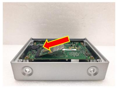
Step 5 Press it down gently, but firmly, and then secure the PCI Express mini card to the carrier by tightening up the one M2 Phillips screw to the marked position.
