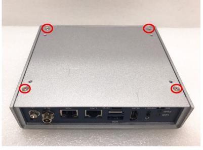
Step 3 Remove the bottom cover, and locate PCI Express mini card slot on the board.
