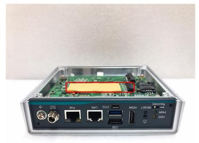
Step 6 Holding the M.2 2280 Key M SSD drive at a 30 degree angle up from horizontal, slowly insert the golden fingers into the M.2 2280 Key M slot until it is fully inserted in.
