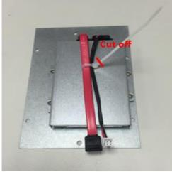
Step 5 Connect SATA+Power HDD cable to the board connector, SATA side first then power side second.
