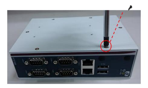
Step 3 Loosen 4pcs screws of the cover, and put the HDD into the HDD bracket and fix the HDD by 4pcs of screws in the accessory bag.
