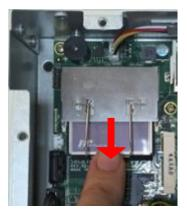
Note: Unlock the CF card from the socket and pull out the CF card when taking out CF card.
